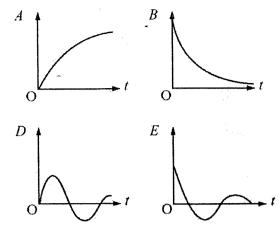
Select the graph that most nearly shows the nature of the time dependence of the voltage across the inductor in the circuit after the switch is thrown.
